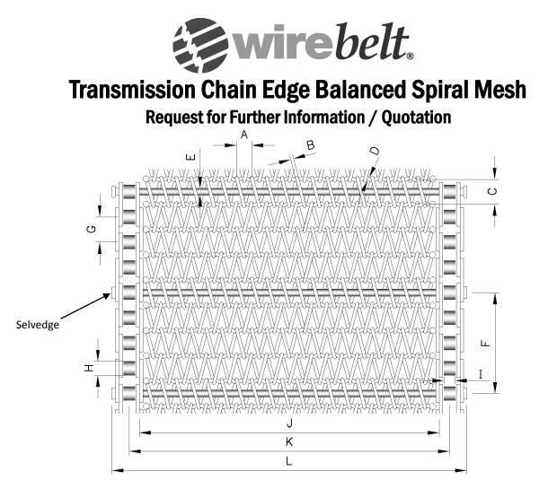
\*NOTE: When measuring pitches A & C, it is best practise to measure over 10 pitches and then divide by 10 to obtain the average pitch.
