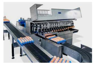
After the arrival of the 6th egg in the dropset, the Farmpacker places all the eggs into a tray in one cycle. The result of the concept of individual egg handling is:
