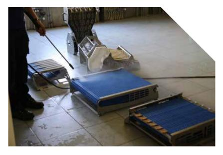
All the egg-touching parts of the Mopack150 can be removed from the machine for cleaning outside egg packing room. The main advantage of this construction method is that this allows for a hygienic and clean packing process. This will ultimately result in more grade-A eggs being supplied to your egg retailer.
